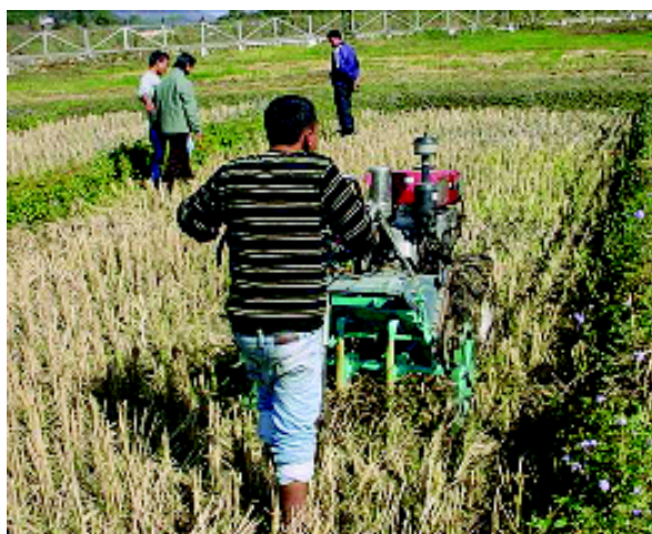
Fig 1 Inclined plate planter in operation
