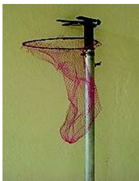
Fig 3 Light weight cutting type fruit harvester
