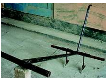
Fig 7 Adjustable zero till furrow opener
