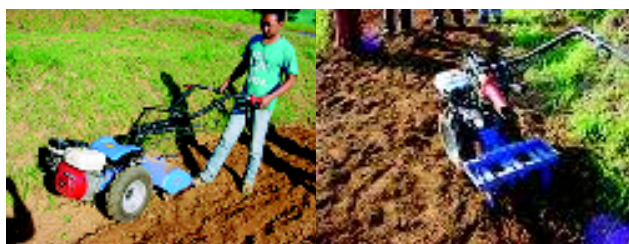
Fig 8 Lightweight power tiller with different attachments
